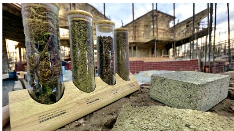
Photo 4: The Waste2Build solution from BSF Innovation Limited uses green powder produced with food waste and black soldier fly in bricks and can reduce 60% of greenhouse gas emissions as compared with traditional building materials.
