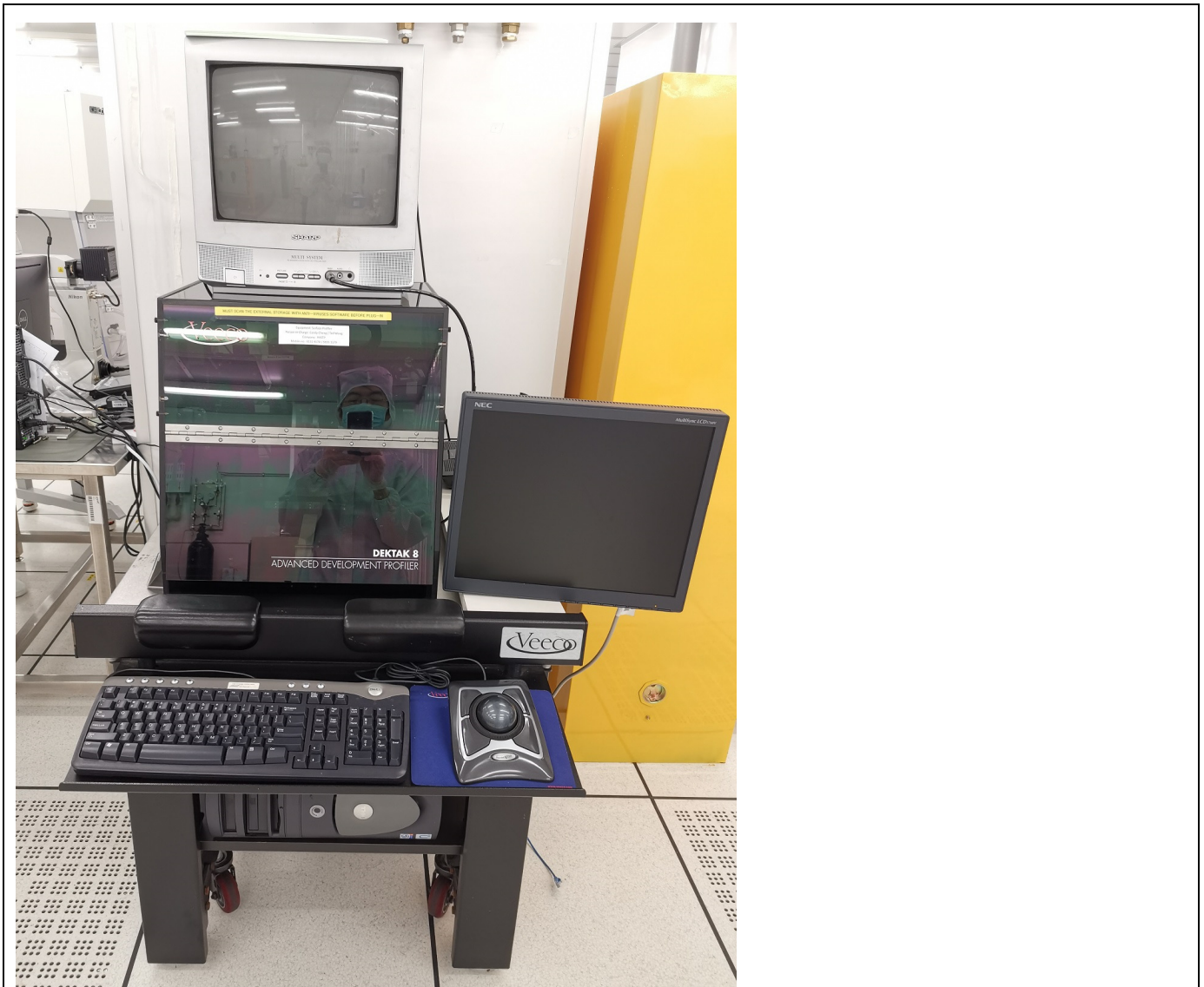
Figure 1: Veeco: Surface Profiler S/N: 23142 (SPIL000020) Power Adapters for Surface Profiler (SPIL000021) Power Adapters for Surface Profiler (SPIL000022) PC - Dell Linux Workstation – 2 (SPIL000023) PC - Dell Linux Workstation – 3 (SPIL000029) (For reference only)
